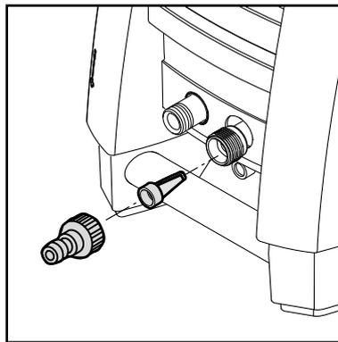
1. Screw the quick coupling tight on to the water inlet (2).
