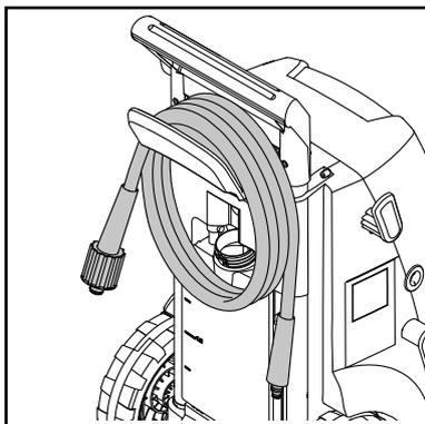
To avoid accidents, the electric cable and the high pressure hose should always be wound
