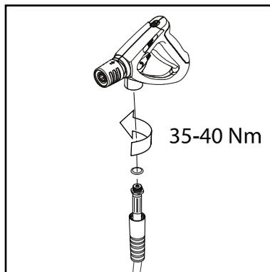
Attach the high pressure hose (4) to the spray handle (7).
