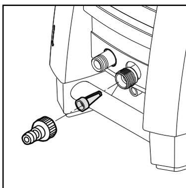
Clean the water inlet filter regularly once a month or more frequently according to use. Carefully loosen the filter with a pair of pliers and clean it. Check that it is intact before re-mounting it.
