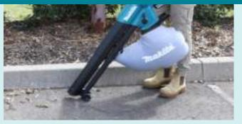
Front wheels allow for single hand operation by taking the weight away from the user
