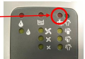
Refill the tank with water and wait until water is boiled and the green “Steam Ready” indicator light turns on. If topping up water after using the machine for a while, the “Steam Ready” indicator light will turn on almost instantly and it is ready for use.
